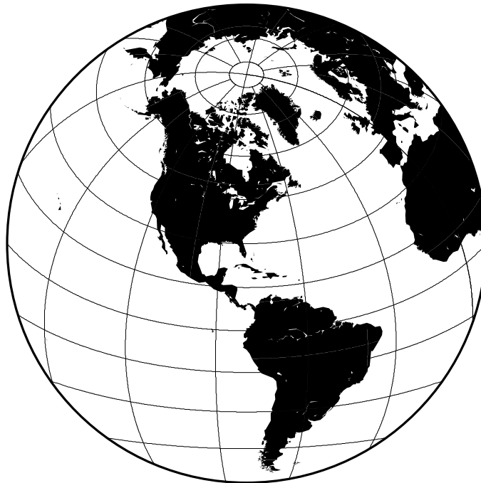
Figure 6.6: Hemisphere map using the Lambert azimuthal equal-area projection.
