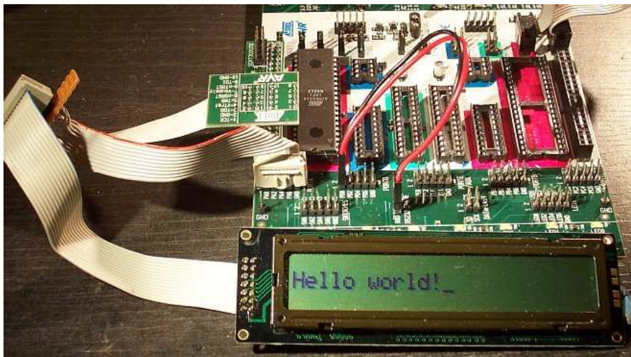
Figure 9: Wiring of the STK500
