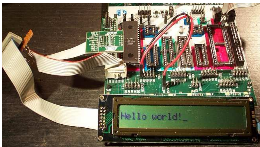
Figure 9: Wiring of the STK500
